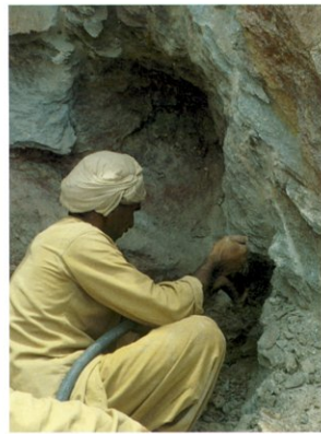
Figure 13. Miners use pneumatic drills to remove the relatively soft host rock at Gujari Killi. Because of the lack of roads, the compressor was carried to the site part by part and then reassembled at the mine. Photo © G. Bowersox.
