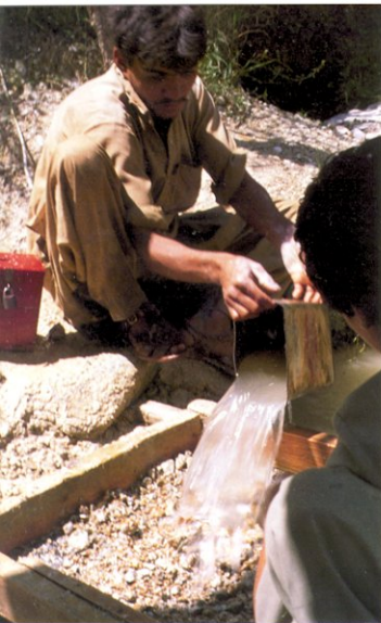
Figure 14. Emeralds are washed from the talc at Gujar Killi before they are sent to the Mingora mine for sorting. Photo © G. Bowersox.
