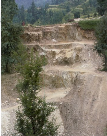
Figure 12. A series of benches characterize the open-cast workings at the Gujari Killi mine. Photo © G. Bowersox.
